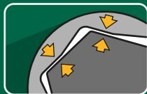
TECNOLOGIA SURFACE DRIVE: EVITA QUE A CABEÇA DO PARAFUSO ESPANE
